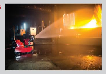
then transmitted live to the operator's control unit, allowing firefighters to assess the fire scene and guide the robot remotely from a safe distance.
