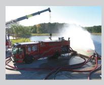
standard industrial rating of 100% capacity at only 100psi (7 bar) net discharge pressure. Breaking the 100-psi ceiling was made possible by the unit's new HPV6000 pump from US Fire Pump. According to Ferrara, with four 8-inch (20.3cm) and one 12-inch (30.4cm) intake connections, the ability to be remotely supplied from mega hydrants is now feasible.
